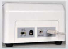
BR-5200 can be connected to a computer via a USB cable.
