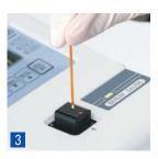
Insert a capillary tube (containing a sample) into the holder.
