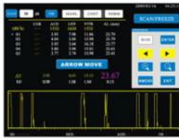
A-SCAN Automatic Reading Automatic measure system, 8 readings for one group. Users can manually adjust the reading results during the automatic measuring
